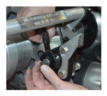
6. Once the gap is set, hold the adhuster bolt and tighten the jam nut.
